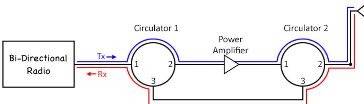
The numbers are good. A single Circulator can have an insertion loss of less than 0.5 dB outgoing with at least 35 dB of rejection for incoming frequencies. A dual Circulator can have 0.7 and 75 dB numbers.
