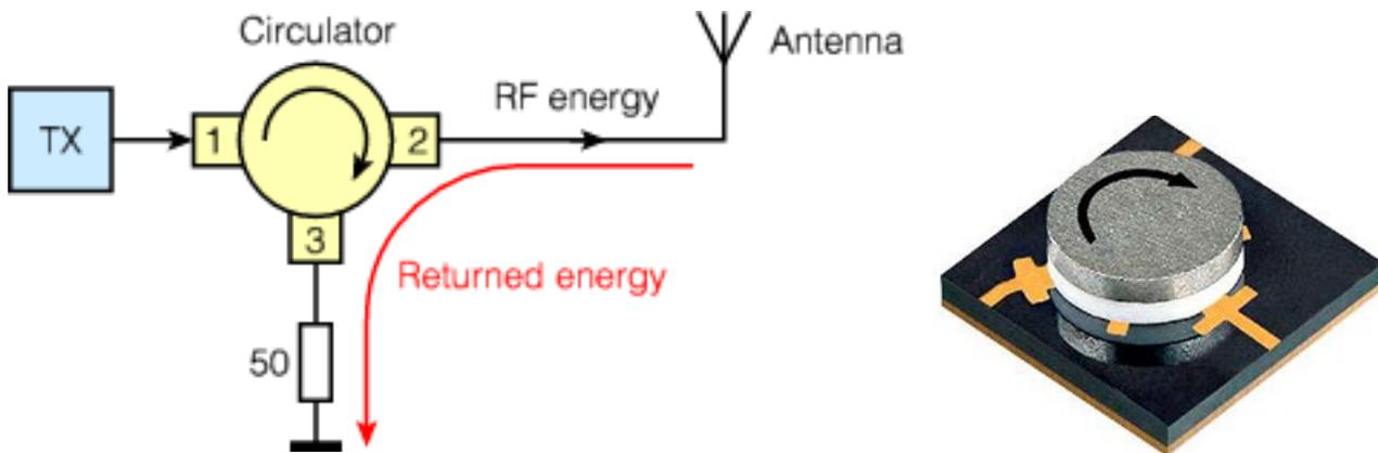
For the JagRF case in point, the Circulator would be placed between the TX and an untuned duplexer. Any untuned duplexer reflects power (presents high SWR). The Circulator would send the reflected power to a dummy load and protect the transmitter or signal source.
